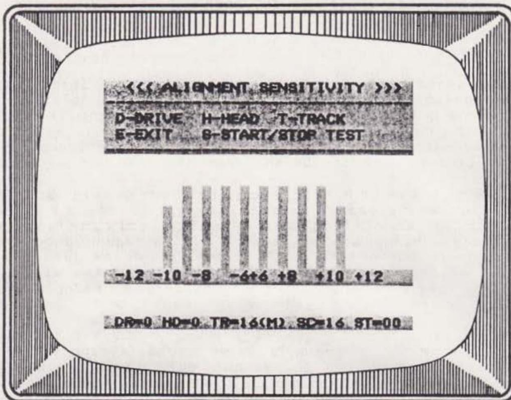
Figure 11: Normal Sensitivity, Proper Alignment
