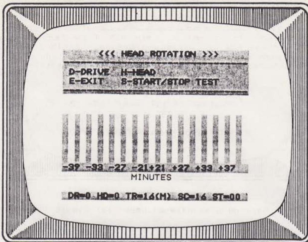
Figure 17: Head parallel to test track
