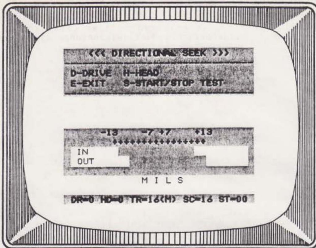
**Figure 16: Poor Directional Seek Results**
