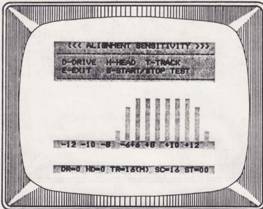
Figure 12: Head Out of Alignment
