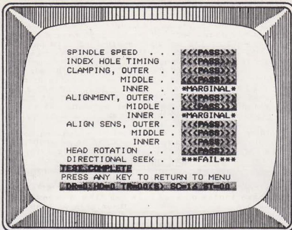
Figure 7: The Quick Test Menu
