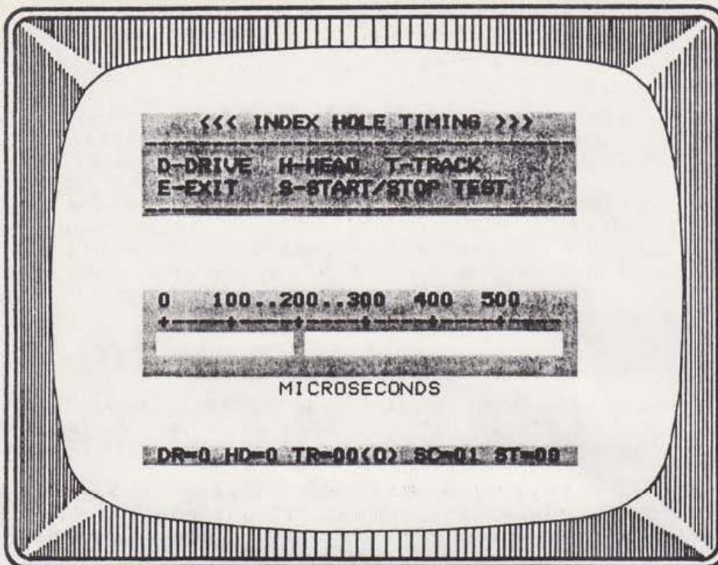
Figure 10: The Index Hole Timing Display
