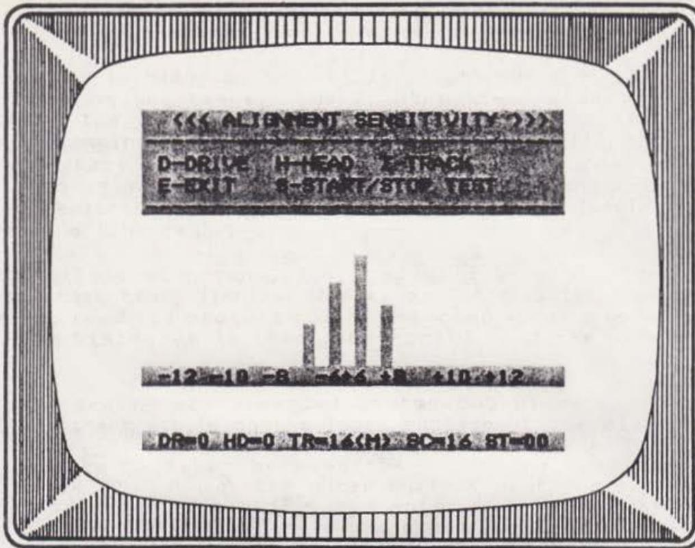
Figure 13: Poor Read Sensitivity
